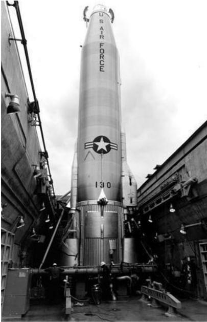
An Atlas E missile being fueled with liquid oxygen and kerosene in 1957.
